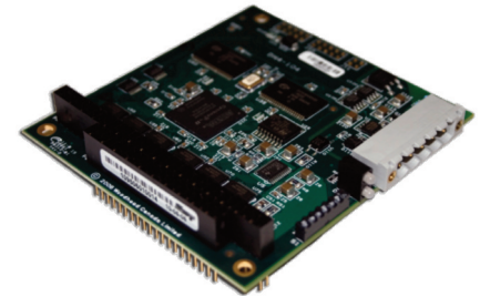
DN4 DeviceNet PC/104 Card Series 112005
